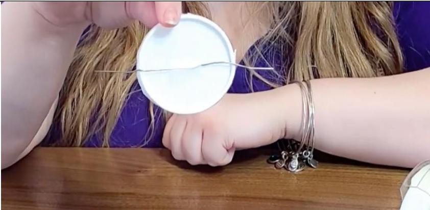
**5. Float your homemade compass in a bowl of water. Watch it rotate. When it starts to settle and finally stops, you'll know that your compass has found north!**
